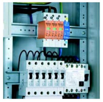
even with powerful surges. Even at a maximum load  $I_{max}$  of 50 kA the protection level is below 1.5 kV. This enables this type of device to withstand even partial lightning currents from direct lightning strikes. In the event of an overload, the built-in isolating device isolates the faulty arrester module from the network and indicates this with a red field.
